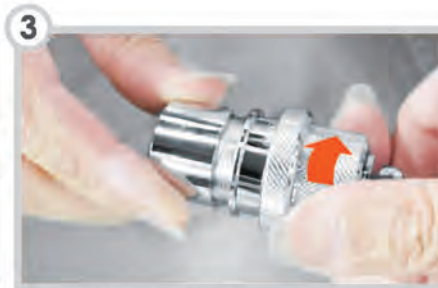
本體與上固定體對鎖，將螺紋順時針方向鎖緊(需轉動本體鎖入，非轉動接頭) The body and upper one are locked together. Screw clockwise and be sure to only rotate the body itself instead of the whole connector.
