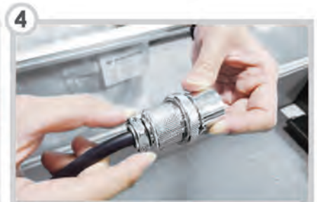
半月邊壓入(與線材不能留有間隙) Crescent-shaped clamp mounted ( The gap couldn't be allowed with the cable connected )
