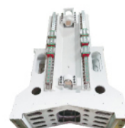
立柱6滑塊 6 Slide blocks on the column
