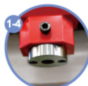
1-4 模頭套筒可依尺寸更換 The size of chuck arbor and sleeve can be changed
